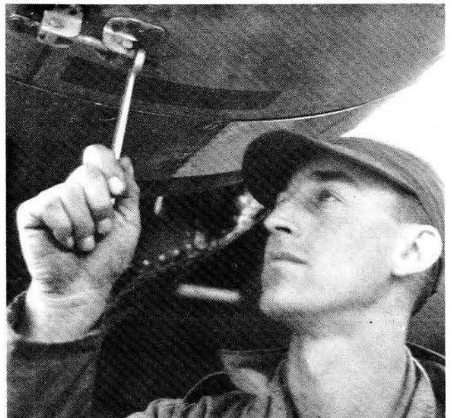
Gotta Haver was the only B-17 with outside fasteners on the engine cowling - Handiwork of Roy Swiler.
